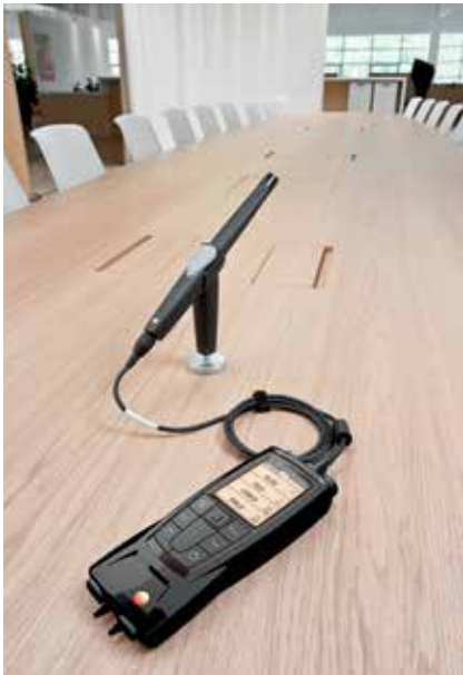
Fig. 13: Measuring indoor air quality using the testo 480.
