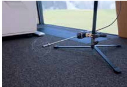
Fig. 8: First draught measurement at a height of 0.1 m on the ground.
