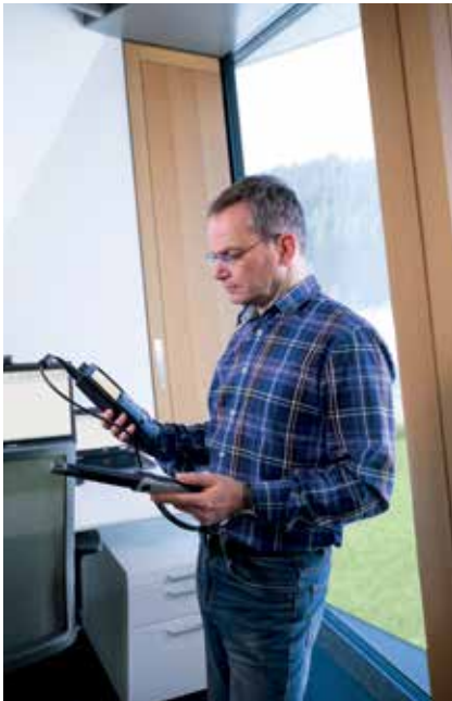
Fig. 3: Measuring the ambient air temperature and humidity using the testo 480 climate measuring instrument.
