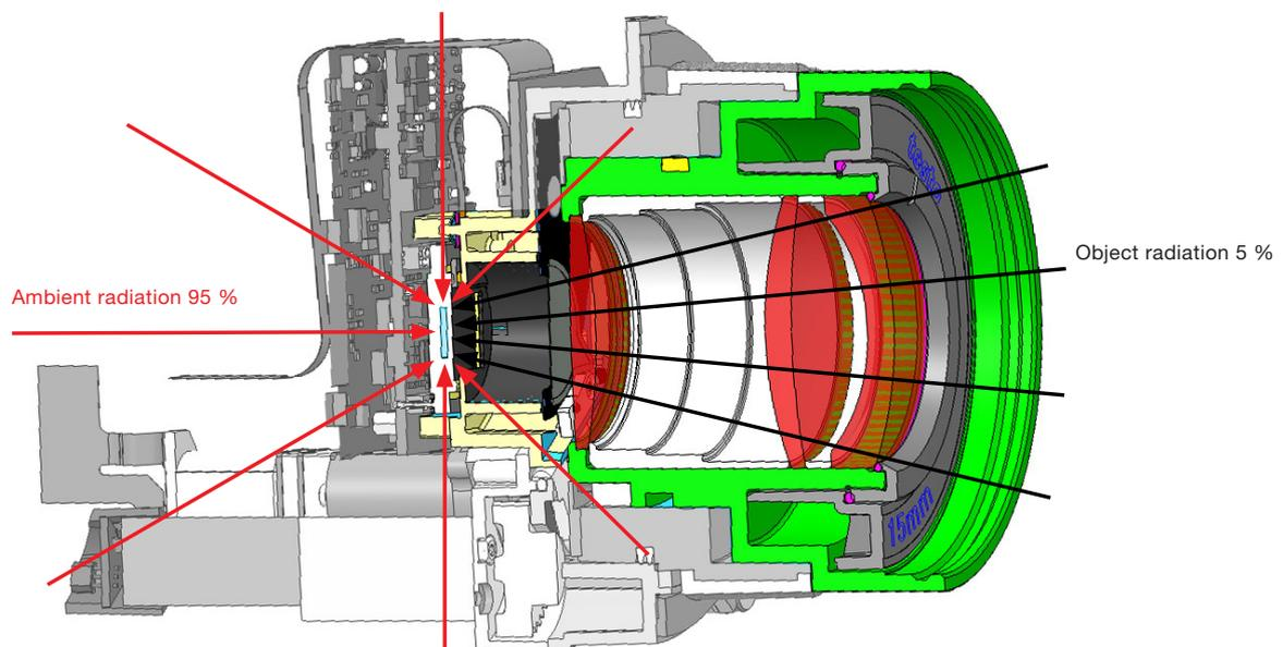
Fig. 1: Cross-section of a thermal imager with detector, optics and electronics.
