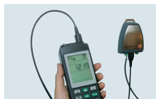
Inspection of transmitters with 4 to 20 mA interface
