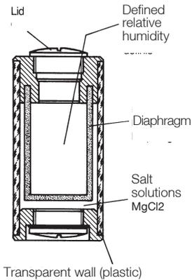
The storage containers are double-walled (see diagram). The inner wall is a diaphragm (porose wall, permeable to water vapour). The outer wall is made of transparent plastic. The saturated salt solution ( $MgCl_2$ ) is located between these two walls. The water vapour penetrates through the diaphragm into the inner part of the storage container and forms an air mixture with a specified water level. This corresponds to a defined relative humidity.
