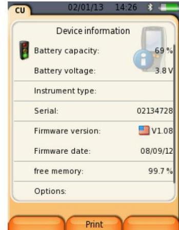
download the firmware update, go to [testo350.com](http://www.testo350.com/testo-350/350-overview.html): <http://www.testo350.com/testo-350/350-overview.html> and check the downloadable firmware version. The version number must be higher than the one listed on the 350 Information screen.
