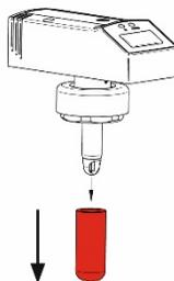
3. Install the sensor in the sealing cone of the measuring station. **Take notice of the correct installation position of the sensor.** Due to the design, the sensor can only be screwed onto the sealing cone in one direction (bolt/groove principle). The head of the sensor, i.e. the display, points in the direction of the inflow. If this is not the case, the measuring station has to be turned between the flanges.
