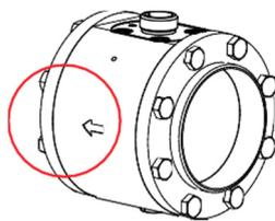
3. Screw the measuring station between the flanges according to the direction of flow. Fix the screws in diagonal order for even force distribution.
