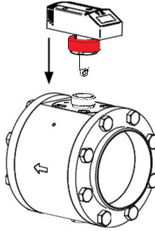
4. Fix the sensor to the measuring station with the union nut **and without tools**.
