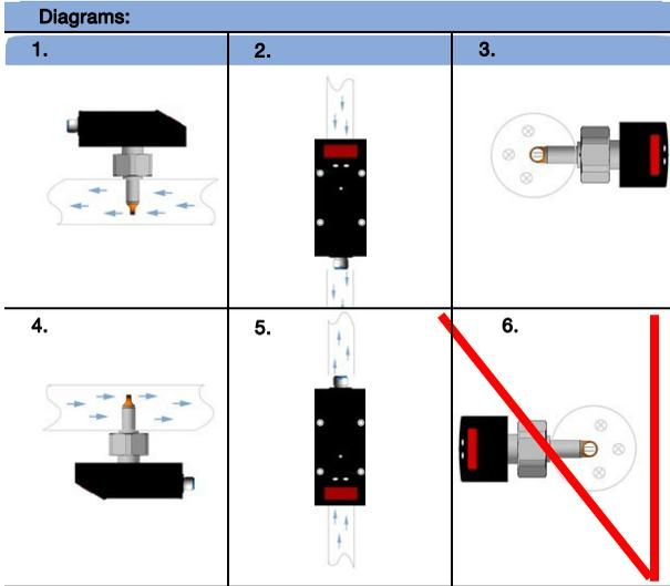
The arrow shows the direction of flow for the medium.
