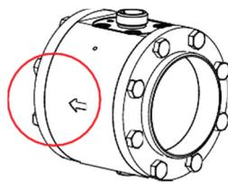
3. Screw the measuring station between the flanges according to the direction of flow. Fix the screws in diagonal order for even force distribution.
