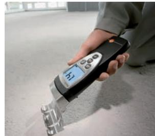
testo 616 measures material moisture non-intrusively using a contact probe in wood, screed, cement and concrete at a depth of up to 5 cm. The instrument simplifies the work of anyone who must observe the drying processes of floors, walls and surfaces as well as moisture damage.
