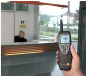
testo 625 measures air humidity, temperature and dewpoint. In inaccessible points such as corners at ceiling height, the measurement values can be transferred wirelessly over great distances by the wireless module to the measuring instrument.
