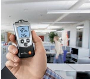
testo 610 is very small and handy, and can be carried with you conveniently at any time. testo 610 is simply held up in the room, and reliably, very accurately and at the touch of a button records the air humidity, temperature and dewpoint.
