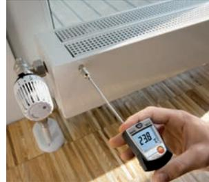
testo 905-T2 adapts itself perfectly even to rough surfaces, achieving a high level of measurement accuracy. This allows the temperature on the surface of a wall, radiator, on valves or connections in a heating system, to be measured quickly.
