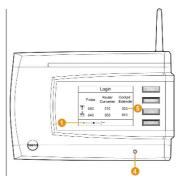
Hold the connect key ② on the rear of the Saveris router pressed down until the LED ③ on the Saveris router starts to flash orange.
